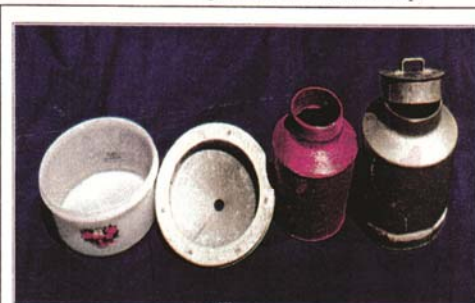
Fig. 2. Exploded view of insect-removal bin. The grain is held in the perforated inner bin (red) and insects can leave the grain and are trapped in the bottom (white).
