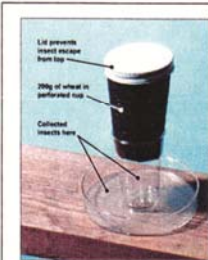
Fig. 1. Cup bioassay to determine repellency or attractiveness of products to stored-product insects. Grain is placed in the perforated container, insects are introduced by a funnel into the centre of the grain mass. Insects leaving the grain are captured in the collection device.
